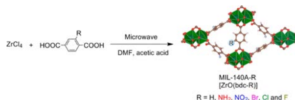
Scheme 1. Synthetic Routes to MIL-140A and MIL-140A-R (R = NH 2 , NO 2 , Br, Cl, and F)
